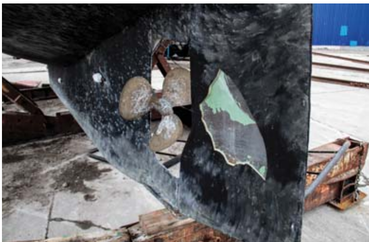
Damage to the steel rudder
